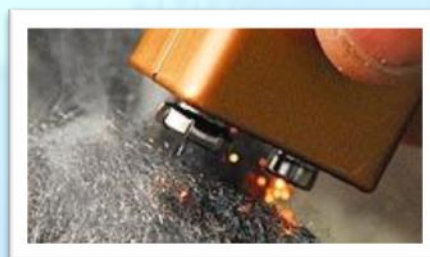
Steel wool begins to burn, sparked by the terminals of a 9-volt battery.
